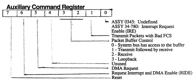
Writing the Reset bit to one resets all control and status registers in the EtherLink adapter. Software must explicitly set this bit to zero after setting it to one. Leaving Reset on has the effect of perpetually resetting the controller.
