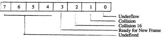
The controller loads the Transmit Status Register only after each transmission or attempted transmission. If interrupts are enabled for transmit, reading the status register clears the interrupt.
