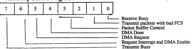
Software starts a DMA transfer by programming the proper channel of the 8237A DMA controller on the system board and setting RIDE, and DMA Request to one on the EtherLink adapter. When the DMA transfer ends, DMA Done goes to one; software clears DMA Done by setting DMA Request to zero.
