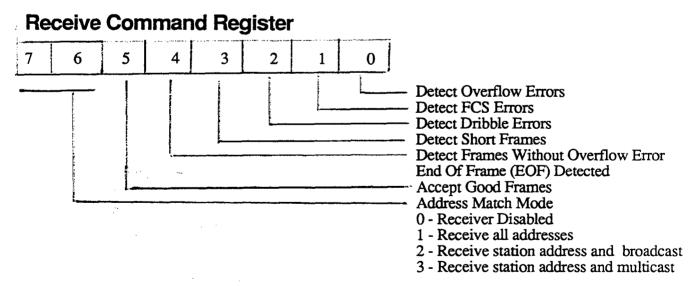
Software can program the EtherLink adapter to detect only certain classes of packets (packets of interest); all unwanted packets are discarded automatically. Discarded packets require no software intervention. After a packet is discarded RP is reset and the controller is enabled to receive the next packet of interest. The EtherLink adapter will generate interrupts on packets of interest only if RIDE and/or IRE (ASSY 34-0780 only) is set.
